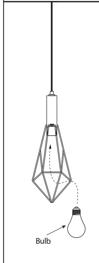
7. Install proper bulb type and wattage (not included).
