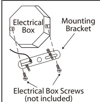
2. Mount the mounting bracket to electrical box using electrical box screws (not included). Make sure the studs on the mounting bracket are facing out from the electrical box.
