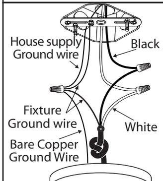
4. Connect the ground wires (bare copper or green) from your fixture to the ground wire (bare copper or green) or ground screw in the electrical box. Connect the black wire from the fixture to the black wire in the electrical box and connect the white wire from the fixture to the white wire in the electrical box.
