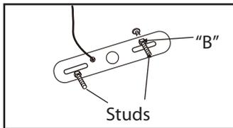
1. Loosen "B". Adjust stud to desired length and lock in place with "B".
