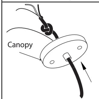
3. **Adjusting the length of flexible cord. For safety, do not release the knot inside canopy.**
