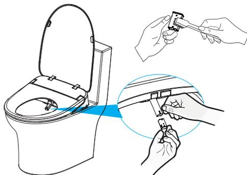
**Tip:** Do not pull the nozzle rod to prevent damage to the nozzle rod and motor.
