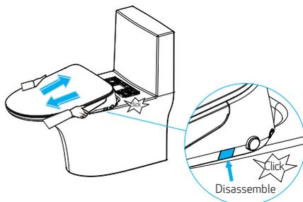
Installation of Main Unit: Align main unit to base plate and push it into the base plate. A "click" sound means that the main unit is installed in place. Removal of Main Unit: Press the "Quick Release button", and pull out the main unit when a "click" sound is heard.
