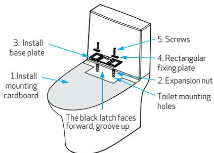
Place the mounting cardboard on the bowl to guide the base plate installation. Install the expansion nuts into the toilet mounting holes first, and then install the base plate, the rectangular fixing plate and then attach with the screws. Attach the base plate loosely until the final positioning of the seat is determined, and then tighten.
