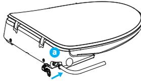
**Installation:** Install the quick release connector of the water inlet pipe into the main unit, and clip the clamp into the slot.
