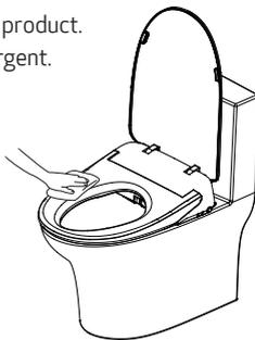
**Tip:** Do not rinse the surface of the product directly with water during cleaning.
