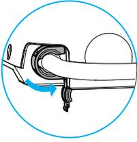
**Removal:** Open the clamp cover, rotate it counterclockwise, and use a flat-head screwdriver to carefully pry the clamp out of the slot.
