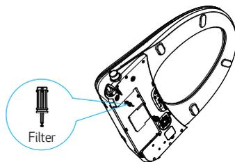
**Tip:** When cleaning, do not lose or damage the sealing ring on the filter assembly and the filter connector, otherwise it will cause water leakage.
